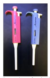
**Figure 2.6** A set of two digital micropipets. The pipet on the left deliver volumes between 0.5  $\mu$ L and 10  $\mu$ L and the pipet on the right delivers volumes between 10  $\mu$ L and 100  $\mu$ L.
