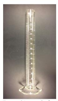
**Figure 2.4** An example of a 250-mL graduated cylinder.
