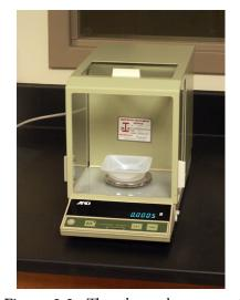
**Figure 2.3** The photo shows a typical digital electronic balance capable of determining mass to the nearest  $\pm 0.1$  mg. The sticker inside the balance's wind shield is its annual calibration certification.
