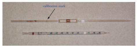
**Figure 2.5** Two examples of 10-mL volumetric pipets. The pipet on the top is a transfer pipet and the pipet on the bottom is a Mohr measuring pipet. The transfer pipet delivers a single volume of 10.00 mL when filled to its calibration mark. The Mohr pipet has a mark every 0.1 mL, allowing for the delivery of variable volumes. It also has additional graduations at 11 mL, 12 mL, and 12.5 mL.
