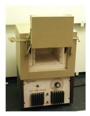
Figure 2.10 Example of a muffle furnace.
