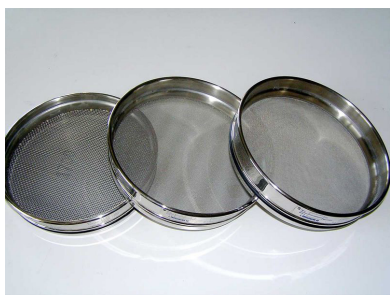
Figure 8.12 Three sieves with, from left to right, mesh sizes of 1700 \mu\text{m} , 500 \mu\text{m} , and 250 \mu\text{m} . Source: BMK (commons.wikimedia.com).
