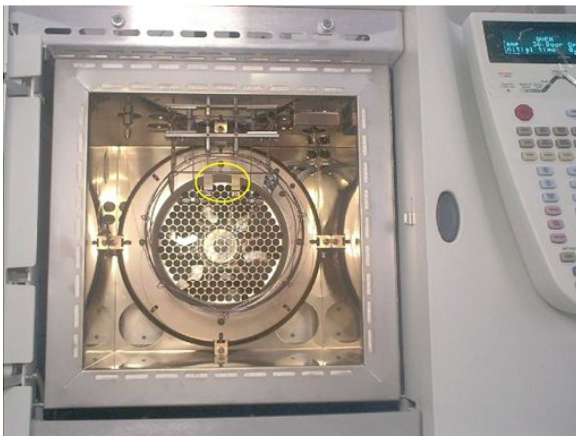
Figure 4.14. Photograph of a GC×GC system with a cryogenic dual-jet modulator.
